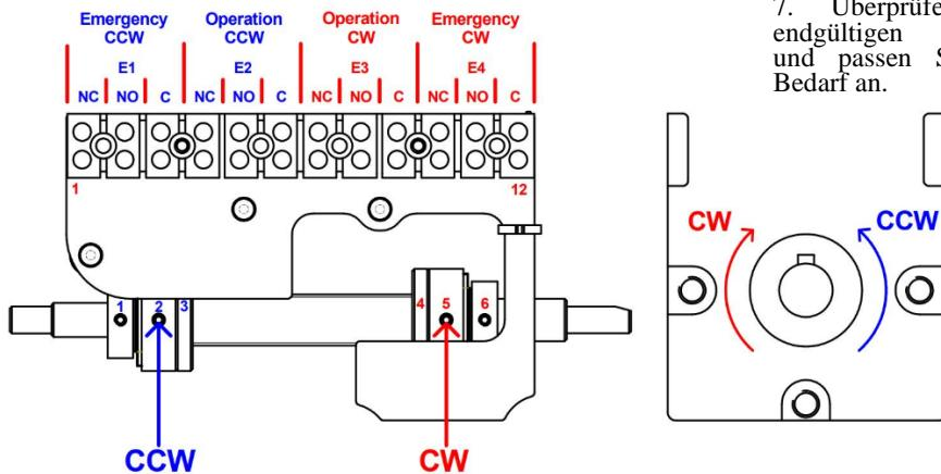
Connect limit switches and electric motor. See junction scheme included as an example.
